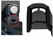
Improved drainage in latch & striker. Sloping features channel water out.
