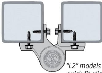
"L2" models have quick-fit alignment legs for fast installation and added fixing strength.
